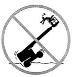
Use extreme care and slow speeds while driving the machine in stowed position across uneven terrain, debris, unstable or slippery surfaces and near holes and drop-offs.
